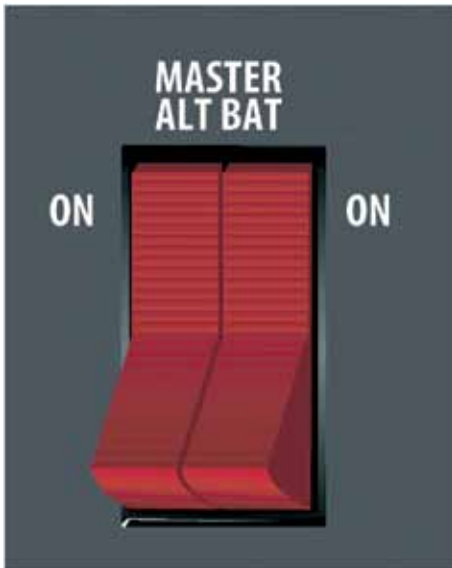
Figura 2.22 – Chave principal – Master Switch
